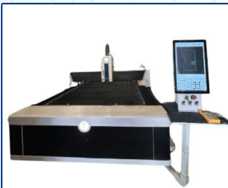
Fiber Laser Cutting Machine 1500W, size: 3mtrx1.5 mtr
